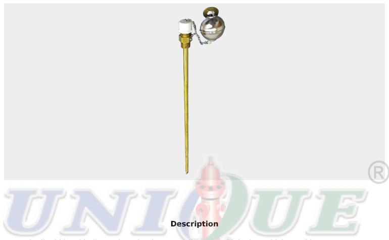
The liquid level indicator is a simple, manually operated device, which provides a means to determine the Clean Agent liquid level in vertically mounted agent storage containers. Once the liquid level is determined, it can then be converted into the weight of Clean Agent present in the agent storage container.
