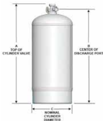
Figure. Dimensions of Cylinder and Valve Assembly, P/N 87-12XXXX-001 Refer to Figure 5-26 for Cylinder Valve details. Table. Cylinder and Valve Assembly Specifications
